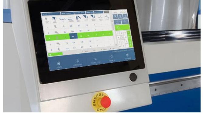
Fastfold Basic CNC line by line software on 15.4" touchscreen controller with swivel arm
