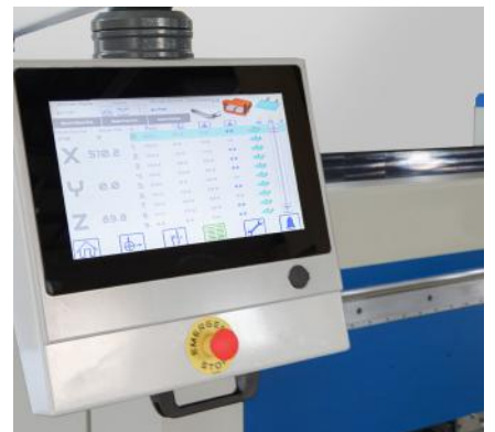
Fastfold Basic CNC line by line control software on 22" touchscreen controller with swivel arm
