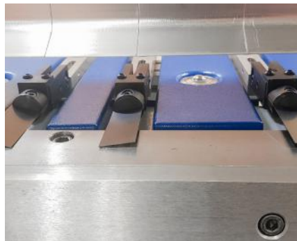
Solid lower beam tool with feather grooves
