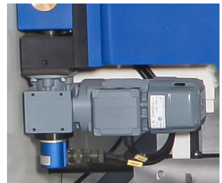
Motorized folding beam adjustment as 80 mm
