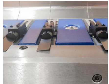
Solid lower beam tool with feather grooves
