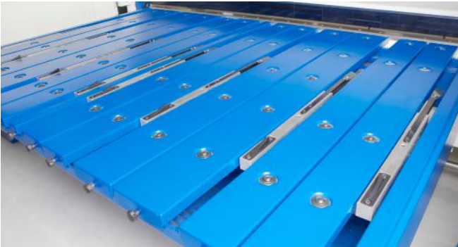
1500 / 2000 / 3000 / 4000 mm motorized back gauge system and sheet support table with ball casters
