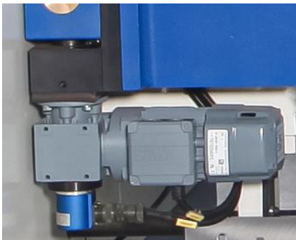
Motorized folding beam adjustment as 80 mm
